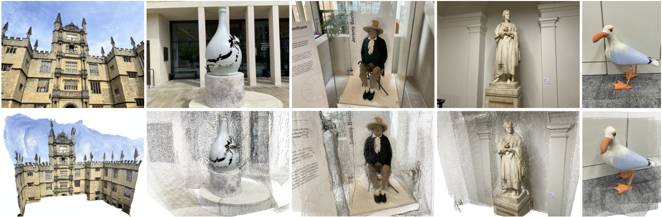
Figure 1. Overview. Given a set of ordered or unordered image collections without prior knowledge of camera parameters, the proposed Spann3R can incrementally reconstruct the 3D geometry by directly regressing the pointmap of each image in a common coordinate system. Spann3R does not require any optimization-based alignment during inference, i.e., the 3D reconstruction of each image can be solved by a simple forward pass with a transformer-based architecture, thus enabling online reconstruction in real-time. The qualitative examples shown are reconstructed from some self-captured images to illustrate the generalization ability of Spann3R.
